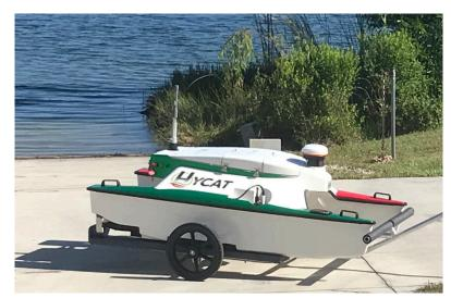
sensors can be installed at any time. Because of this, one HYCAT platform is a perfect solution for habitat mapping, stream gauging, cartography, port inspections, infrastructure inspection, search and rescue, disaster response, volumetric studies, and contamination studies.
